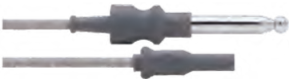
Silicone Monopolar Endoscopic Cable 10" (3.0m) SB-1503 Instrument Connector: 4.0mm Female Plug Generator Connector: Standard Bovie 8.0mm Plug Compatibility: Valleylab, Conmed, Bovie
